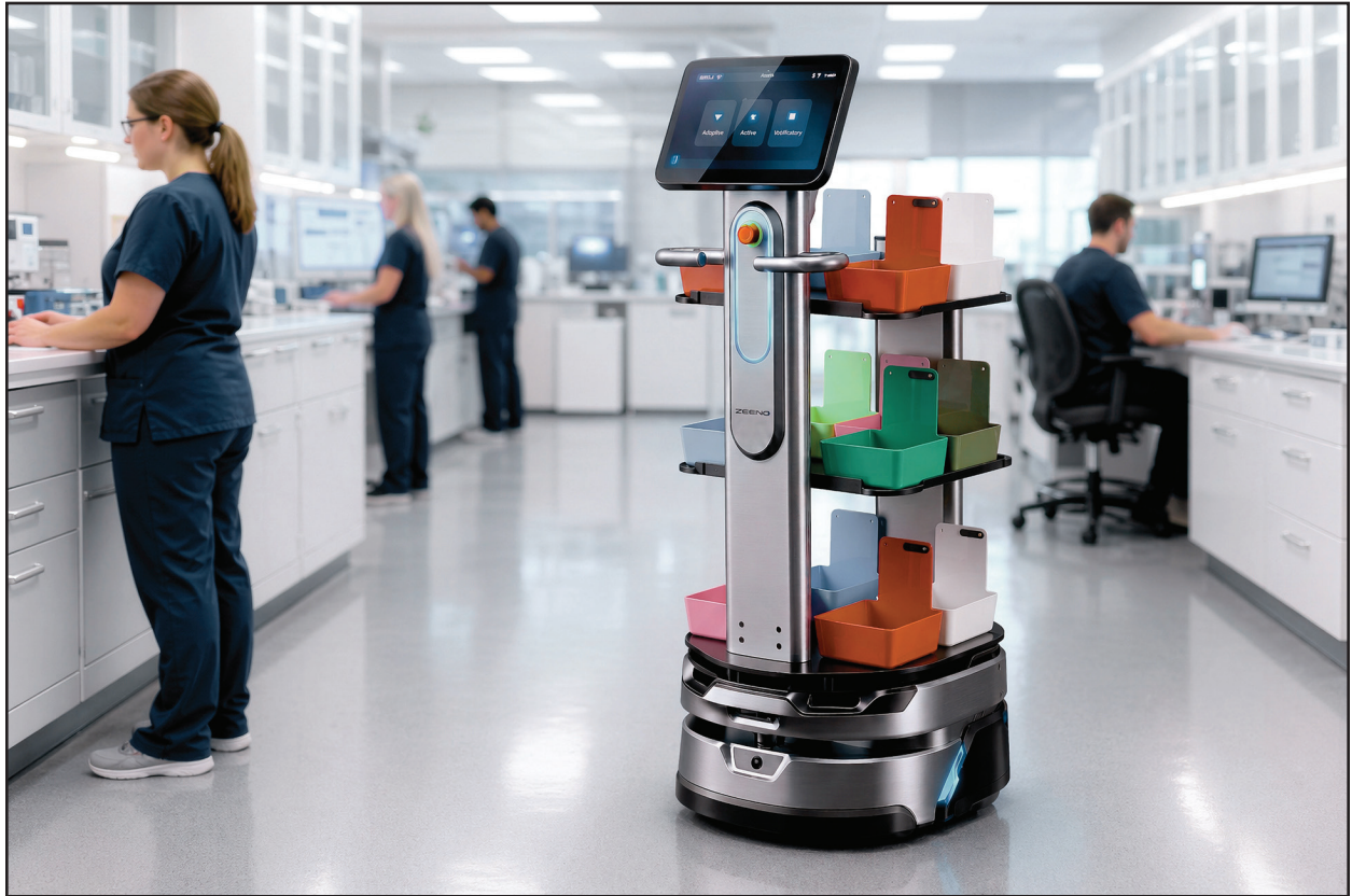
Fig. 4 Digital illustration of Zeeno Carry,* autonomous delivery robot for transporting instrument trays and supplies.
