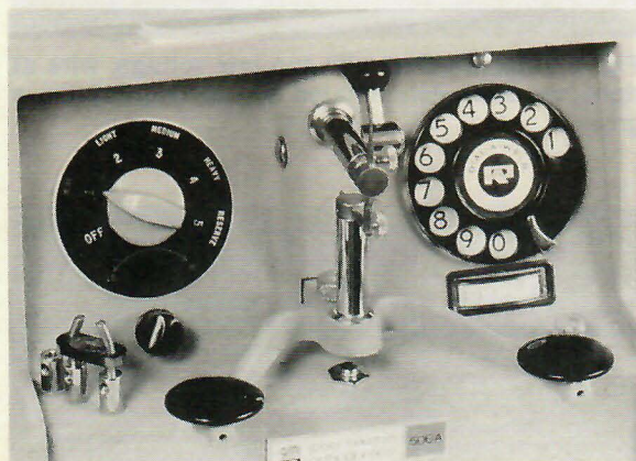
Fig. 1 Rocky Mountain Dial-a-Weld 506A with separate dial indicator showing variable voltage level.
