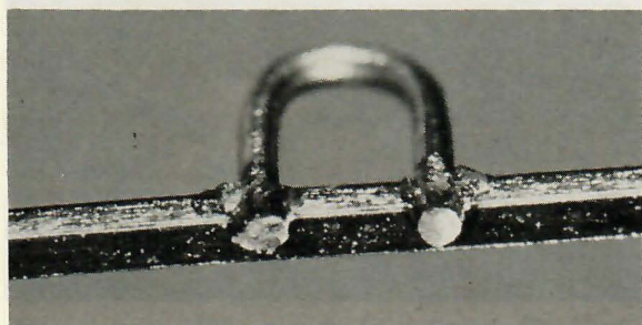
Fig. 7 Overheating causes hook wire to melt and flow, producing potential weakness.
