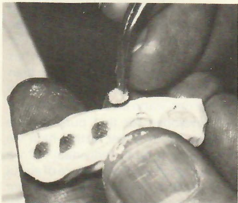
Applying sealant to bracket base.
