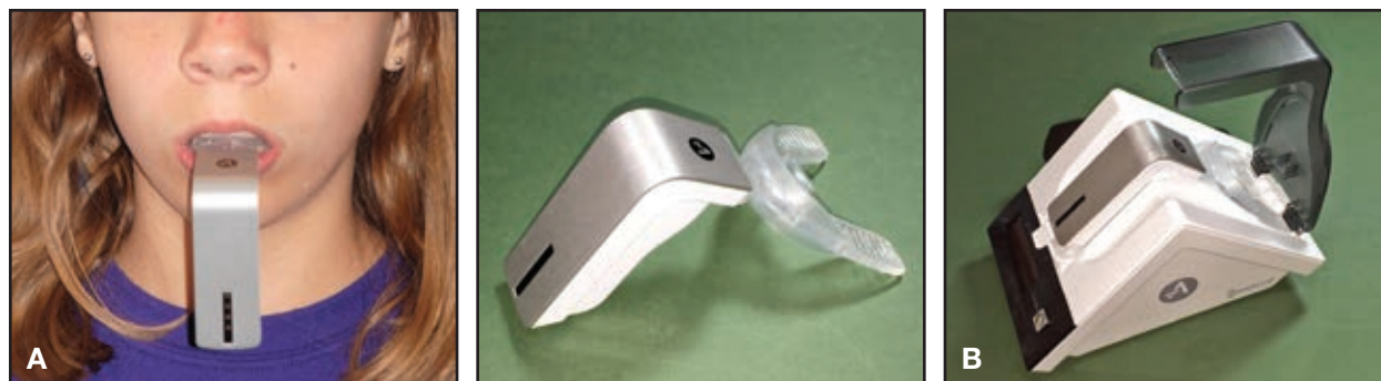
Fig. 1 AcceleDent* device consists of vibrational unit with attached mouthpiece (A) and charging/data-recording station (B). (Note: design has been changed since this study was conducted.)
