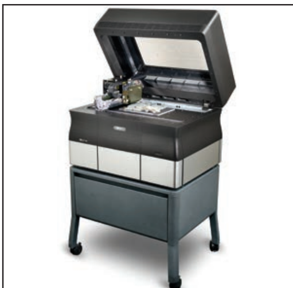
Fig. 6 Objet30 OrthoDesk printer and build area with printed models.
