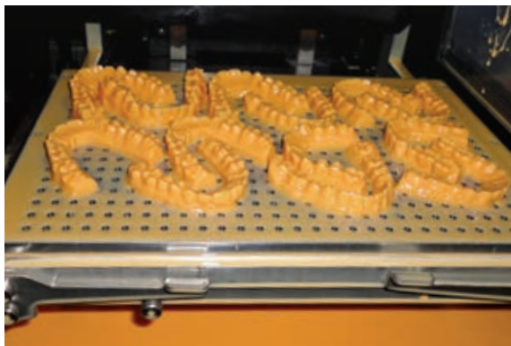
Fig. 7 Ultra 3SP Ortho printer and build area with printed models.
