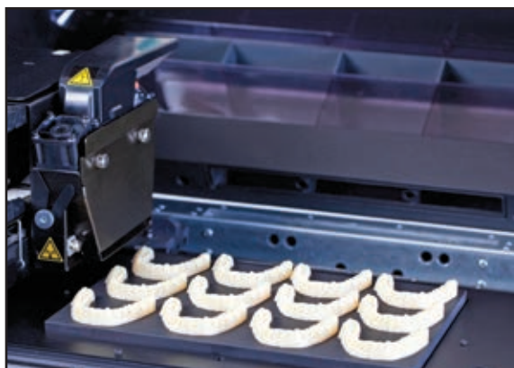
Fig. 6 Objet30 OrthoDesk printer and build area with printed models.
