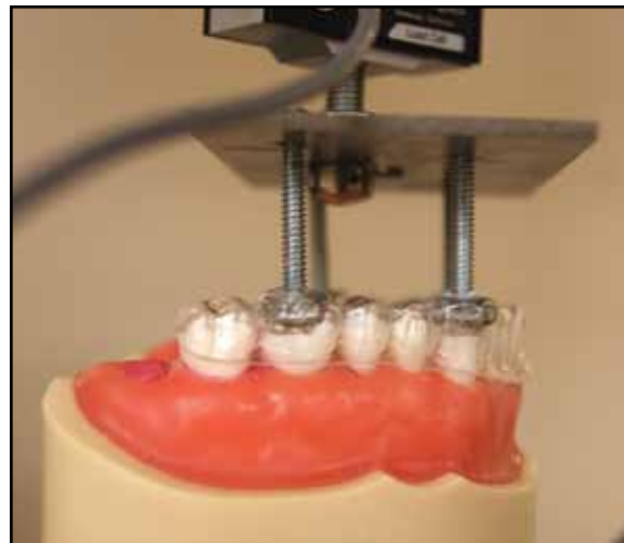
Fig. 2 Pull-off direction on Universal Testing Machine.##
