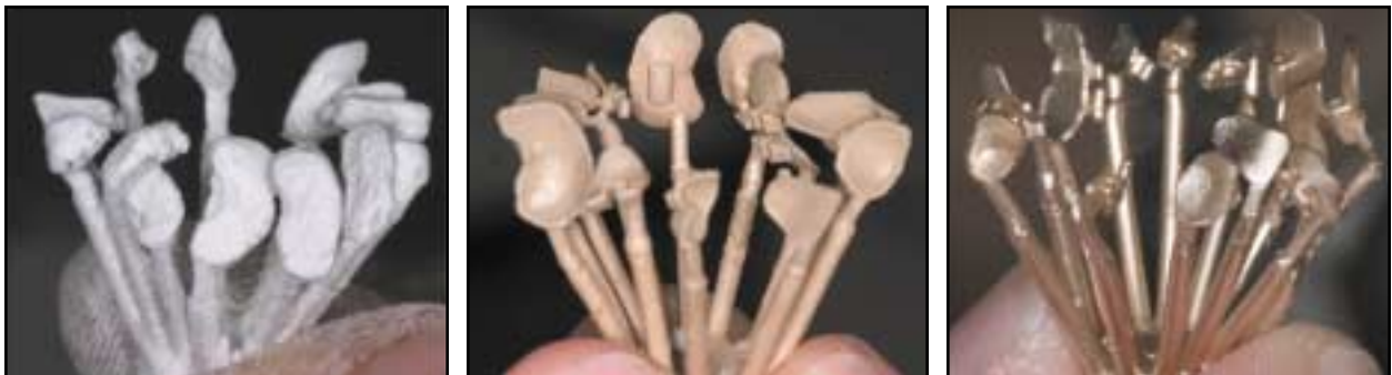
Fig. 10 Brackets cleaned and polished after casting.
