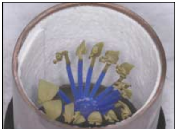
Fig. 9 Brackets with casting spurs assembled in "bouquet" for investment.
