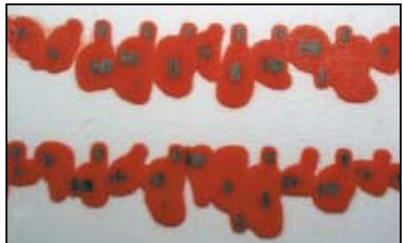
Fig. 8 Virtual bracket series converted to wax analogue.
