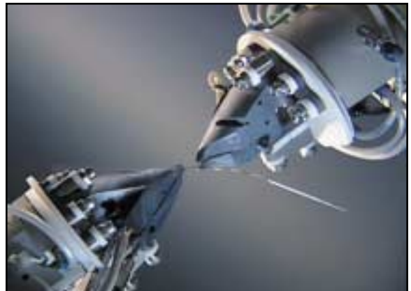
Fig. 14 Customized archwire-bending robot.
