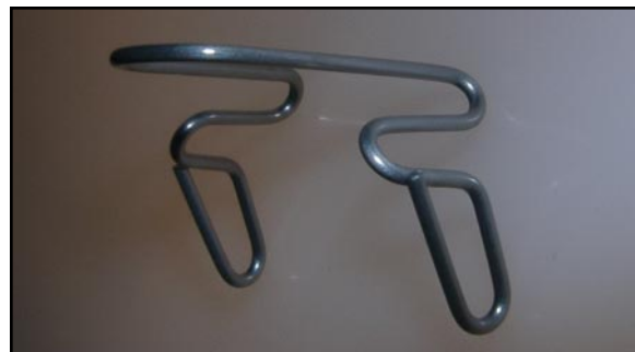
Fig. 12 Prefabricated wire form simplifies appliance construction.
